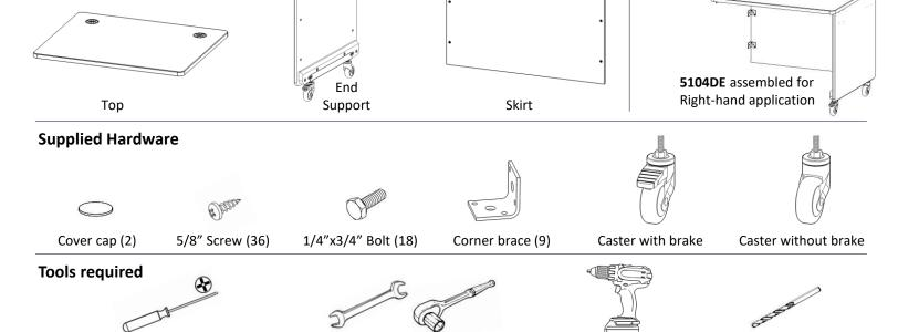
Once it's determined on which side of the main component the 5104DE will be installed on, install hardware to the End Support panel as shown below for Left-hand or Right-hand application.
